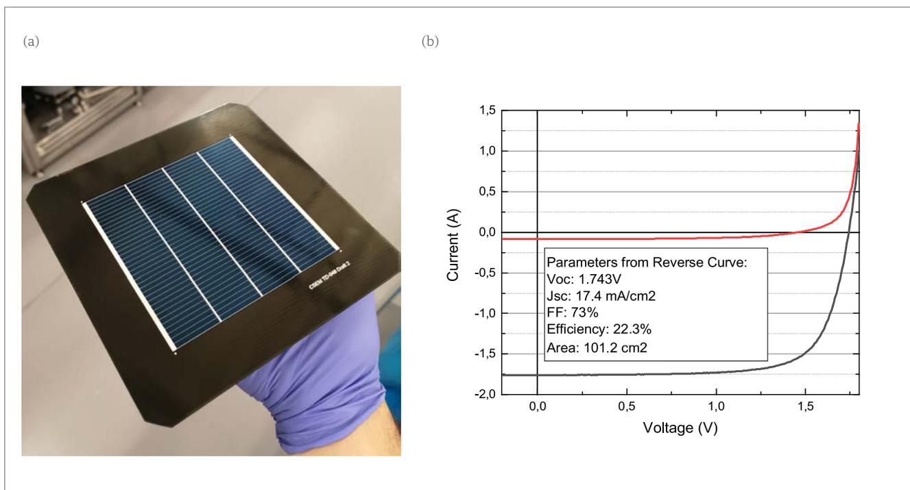
**Figure 1. (a) A 101.2cm<sup>2</sup> PK/Si tandem solar cell built on an M2 HJT bottom cell. (b) I–V curve of the record cell with a stabilized efficiency exceeding 22%.**
