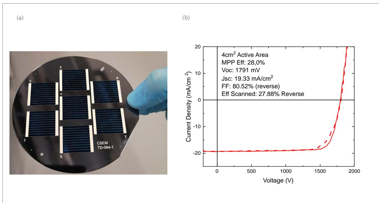
**Figure 2. (a) A 4" FZ wafer with multiple PK/Si devices across its surface, including printed metallization. (b) LIV curve of a 4cm<sup>2</sup> PK/Si tandem with printed metallization, showing a fill factor of over 80% and a stabilized efficiency of 28.0%.**
