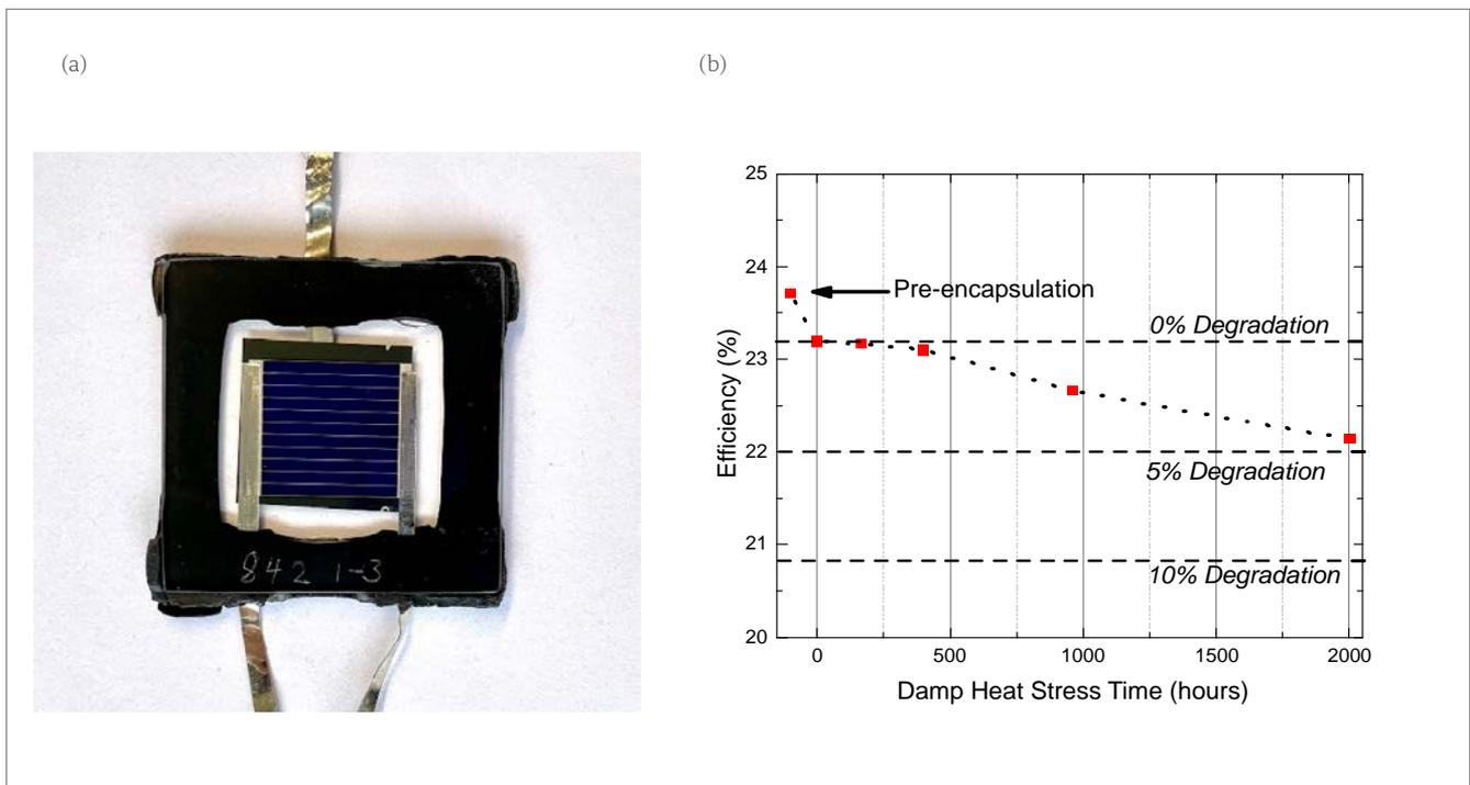
**Figure 3. (a) Example of a 4cm<sup>2</sup> PK/Si tandem solar cell with printed metallization and glass-glass encapsulation with a butyl edge sealant. (b) Damp-heat stress testing of this cell, demonstrating approximately 5% degradation in efficiency after 2,000h at 85°C and 85% RH.**
