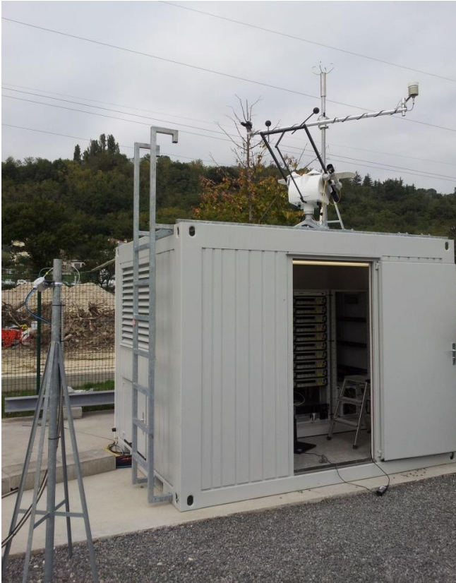
View of equipment container with electronic loads and weather station
