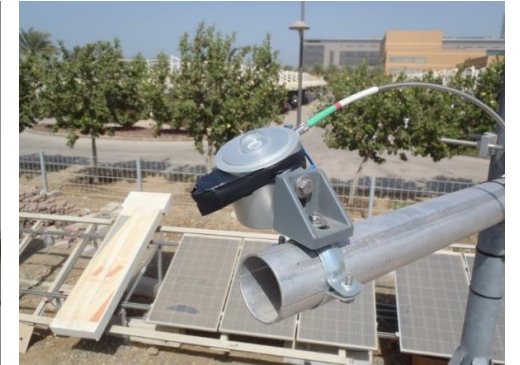
Integrating sphere of spectro radiometer with optical fiber
