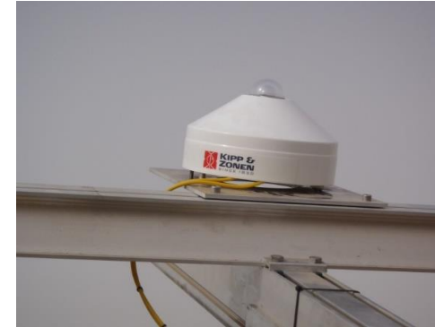
Ventilated pyranometer for measurement of plane of array irradiance
