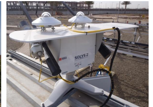
Two-axis solar tracker for measurements of GHI, DHI, DNI
