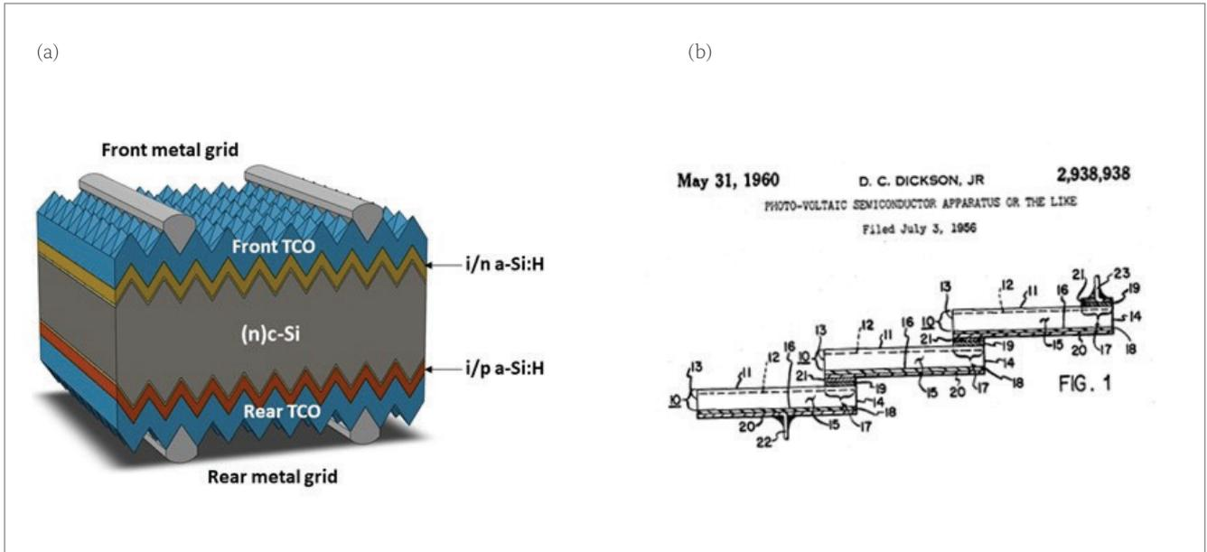
**Figure 1. (a) Schematic of the heterojunction cell device used. (b) Picture taken from a 1960 patent, already describing the shingle concept in use today.**
