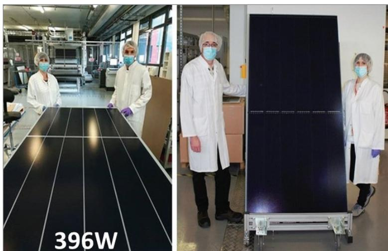
**Figure 12. The two fabricated large-area SHJ shingle modules. Close to 400W was measured for the best module, demonstrating the high potential of SHJ shingle technology.**
