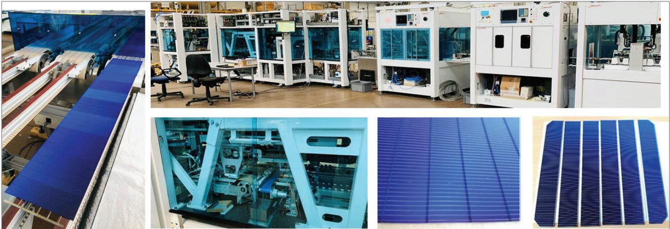
**Figure 8. BSC SONETTO stringer developed by Amat-Baccini, with additional images of the strings produced, as well as of the typical stripes obtained after the cutting of the cell.**
