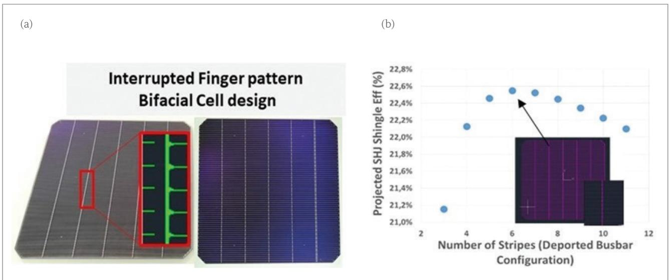
**Figure 2. (a) Photo of a fabricated SHJ shingle cell, with a schematic of the specific busbar and interrupted finger design. (b) Optimization of SHJ shingle tile length, to reach a compromise between metal resistance and cut-edge impact.**
