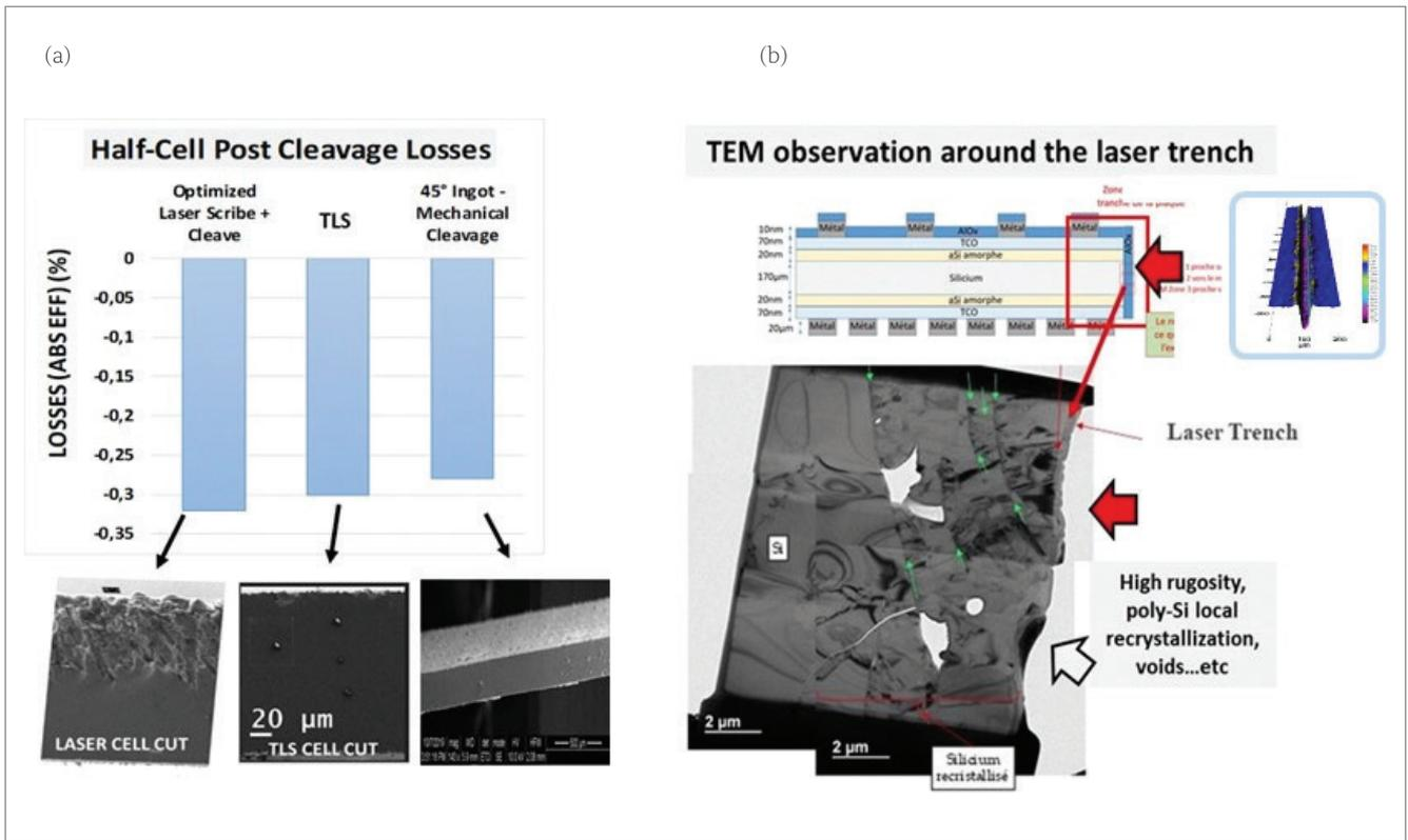
**Figure 6. (a) Comparison of different cutting techniques. If very similar performance losses are observed, the final cut-edge morphology shows a smooth appearance for the TLS and 45° ingot approaches. (b) Strong degradation of both active layers and silicon bulk around the laser trench is confirmed by local transmission electron microscopy (TEM) observations.**
