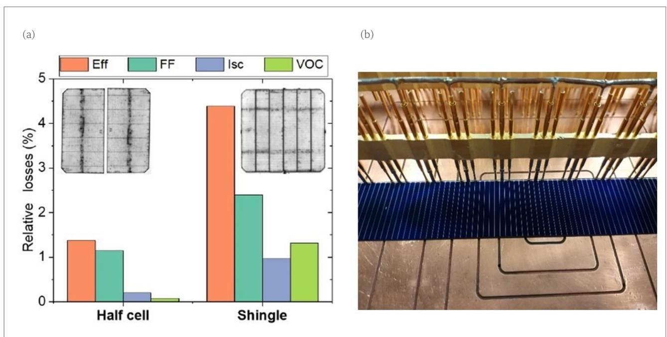
**Figure 5. (a) Typical efficiency losses measured after cell separation for half-cell and shingle configurations. (b) The measurement set-up for an isolated shingle tile.**
