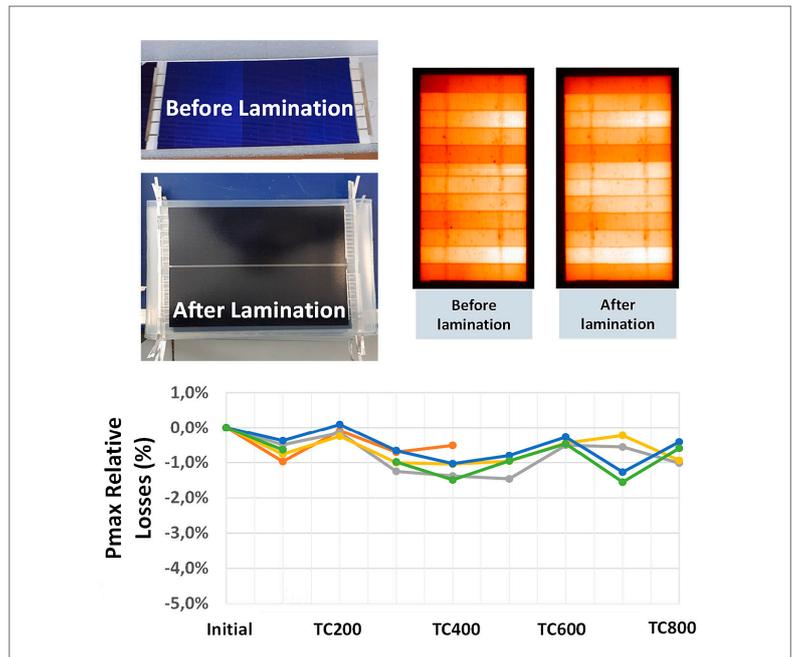
Figure 9. Example of SHJ technology development undertaken at the mini-module level. Outstanding reliability was obtained, and no evidence of cell breakage or degradation was observed during the lamination step.
