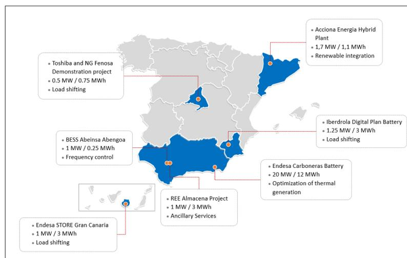
**Figure 11. Operational utility-scale battery storage systems in Spain [1]**
