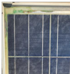
Damaged PV module from the field with evidence of bubble corrosion and delamination.
