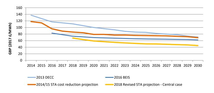
Survey of STA members (Dec 2018) suggests that the median LCOE for large-scale ground mount PV will be 35% lower by 2030 than we had predicted in 2014.
