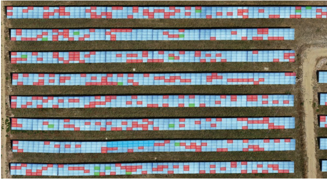
Thermal analysis reveals extensive signs of hot spots across the plant.
