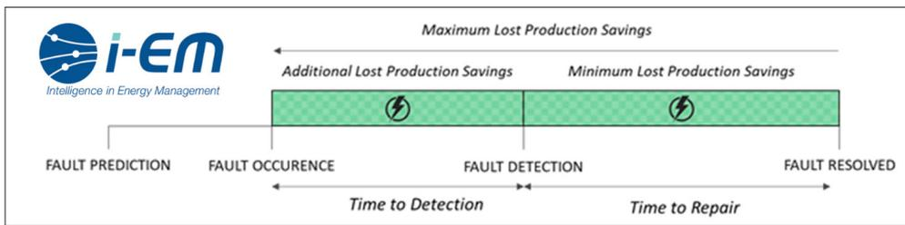
**Figure 9. Fault events timeline. The positions of fault prediction by the predictive service, as well as the fault occurrence, fault detection by standard monitoring platform and nominal behaviour restored are shown. The predictive service allows a lost production saving from one month (assumed as the mean duration of time to repair) up to almost two months (assuming three weeks as the mean duration of time to detection according to current monitoring systems)**
