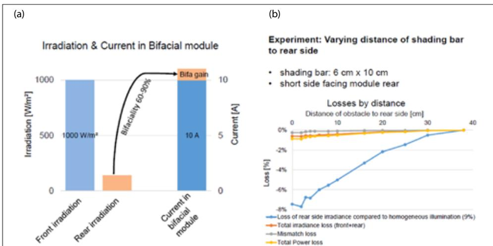
**Figure 6. Hanwha Q CELLS' explanations at bifiPV2018: (a) why shading on the rear side does not cause hot spot problems; and (b) when the shading object is a certain distance from the cell then the shading effect is negligible [44].**
