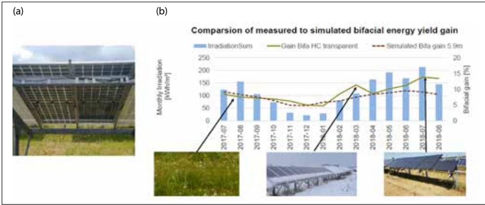
**Fig. 7: Hanwha Q-cell's (a) sub-construction and (b) a graph of monthly bifacial gains in that bifacial PV system [44]. Note: this non-optimal standard sub construction was used on purpose to demonstrate that even in this case bifacial gains of 9% in average were obtained.**
