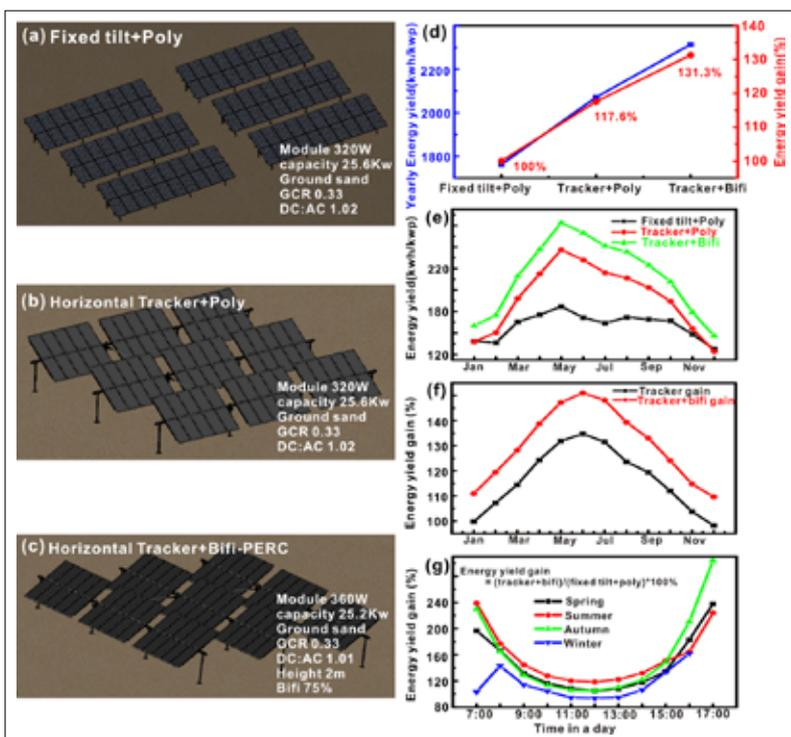
**Figure 2. The energy yield of a poly-Si fixed-tilt system, a poly-Si horizontal tracker system and a bifacial-horizontal tracker system, and the energy yield gain of different systems at different times compared to the poly fixed-tilt system**
