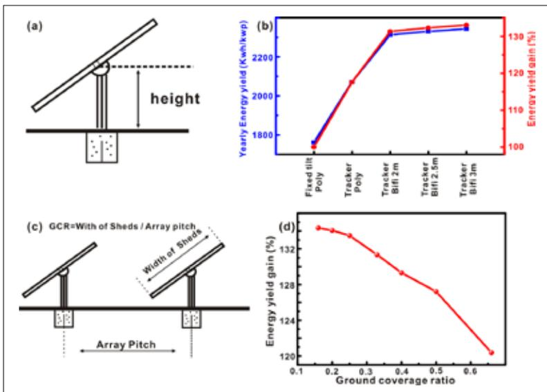
**Figure 3. The energy yield gain of bifacial-tracking system varies with the module height and the ground coverage ratio**
