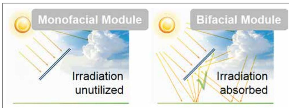
Figure 1. Working mechanism of bifacial modules
