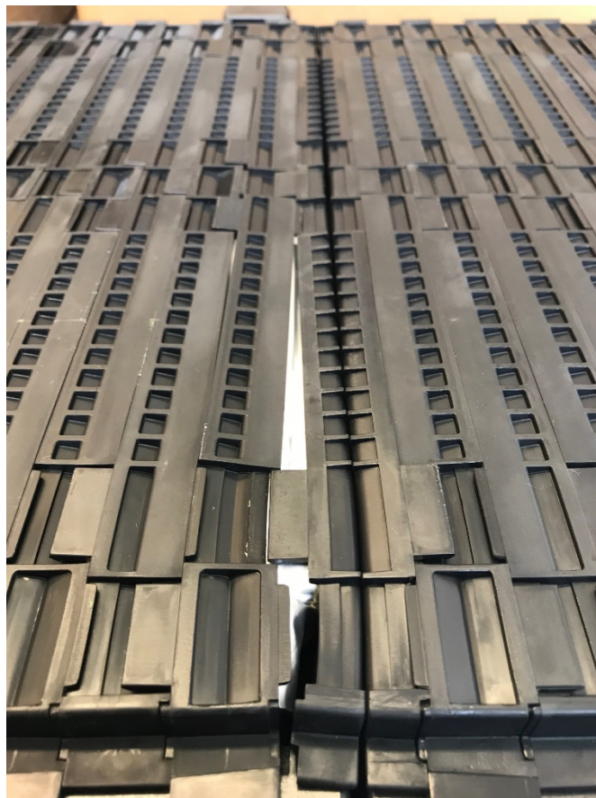
Swollen cells discovered inside the battery module
