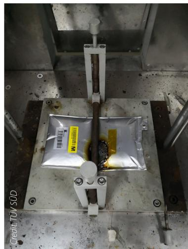
**Figure 4. Cell burning during impact test**
