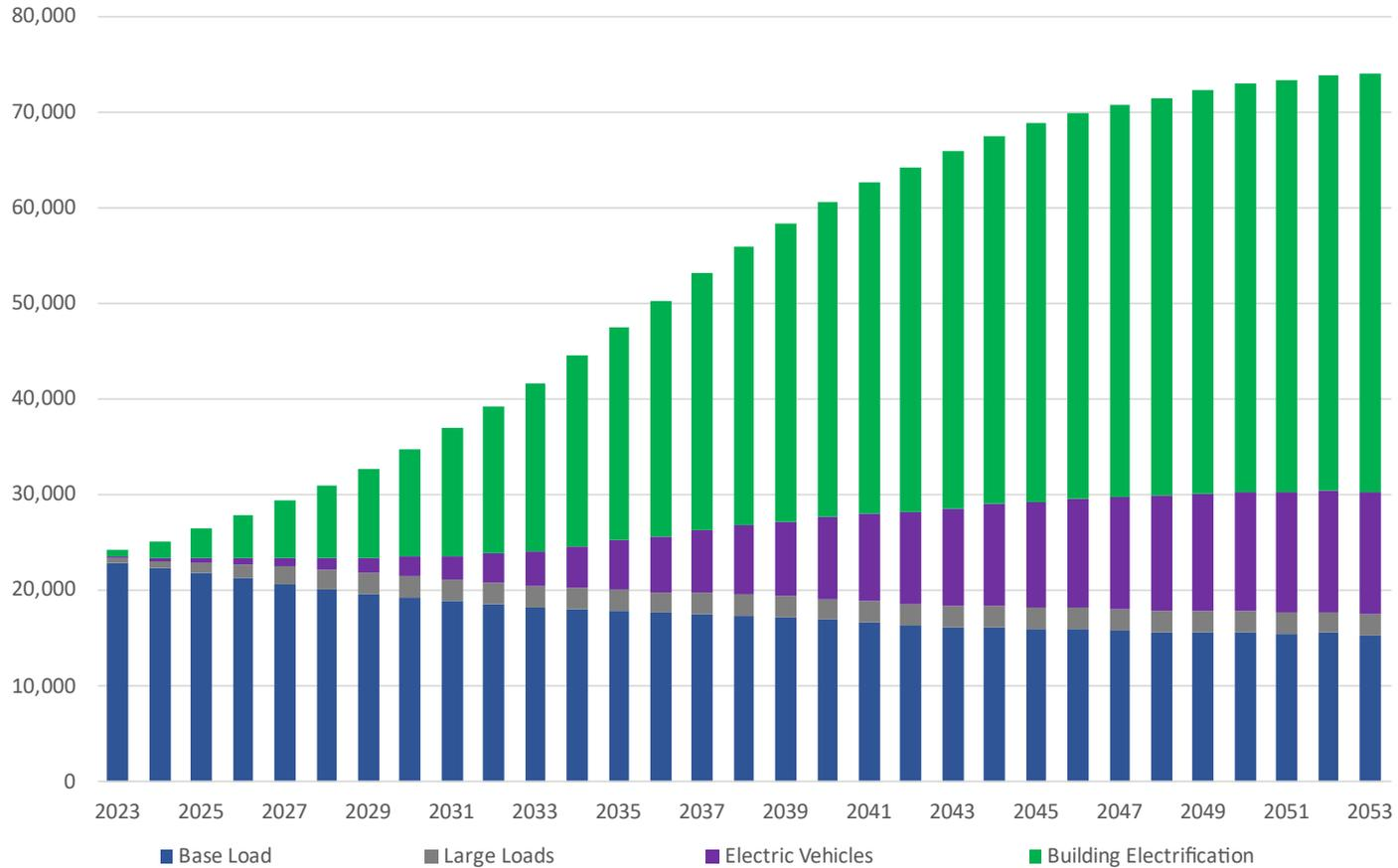
Note: Base load growth includes reductions due to BTM distributed generation, BTM energy storage, energy efficiency, and temperature trends.
