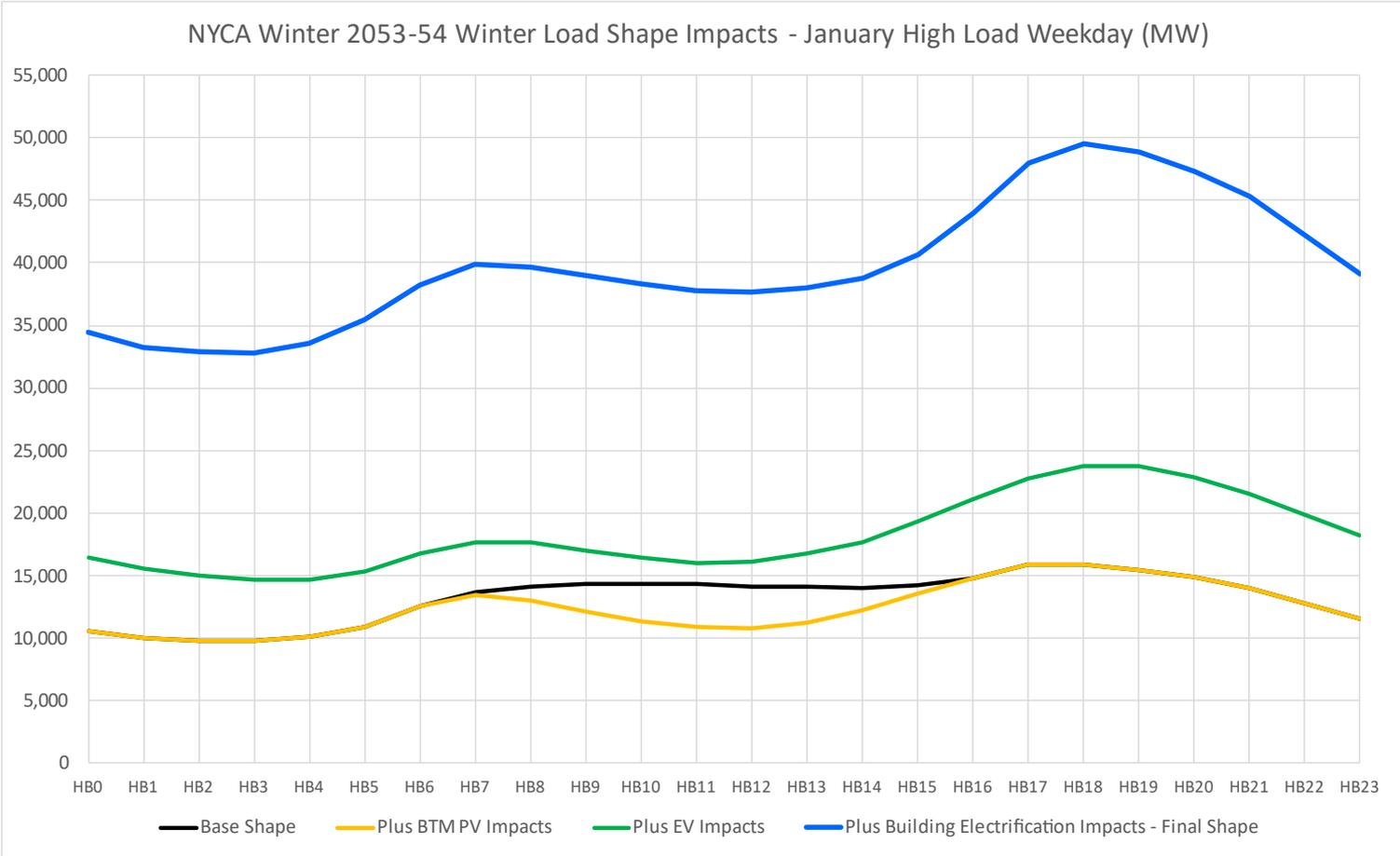
**Black line** shows projected base load shape (gross load).
