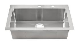
**453-9-RCTM** Square Corner Stainless Steel Topmount Single Bowl Sink Material: T-304 Stainless Steel 18 Gauge Satin Finish Stone Guard Undercoated Overall Size: 33" x 22" x 9" Bowl Size: 29" x 16" x 9" Depth: 9" Sink Weight: 35 lbs. Template and Fastener Clips Included
