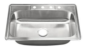
**453-4** Stainless Steel Top Mount Self-Rimming Double Bowl Sink Material: T-304 Stainless Steel 20 Gauge Satin Finish Stone Guard Undercoated Overall Size: 33" x 22" x 9" Bowl Sizes: 27 3/4" x 16" x 9" Each bowl is equal size Depth: 9" Sink Weight: 20 lbs. Template and Fastener Clips Included
