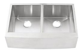
**444-UM-FS** Stainless Steel Apron Double Bowl Undermount Sink Material: T-304 Stainless Steel 16 Gauge Satin Finish Stone Guard Undercoated Overall Size: 32-7/8" x 22-1/4" x 10" Bowl Sizes: 14-3/4" x 17-7/8" x 10" Bowls are the same size Depth: 10" Sink Weight: 35 lbs. Template and Fastener Clips Included
