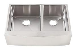
**468-UM-OS-FS** Stainless Steel Apron Double Bowl Undermount Sink Material: T-304 Stainless Steel 16 Gauge Satin Finish Stone Guard Undercoated Overall Size: 32-7/8" x 22-1/4" x 10" Left Bowl Size: 16-3/4" x 17-7/8" x 10" Right Bowl Size: 12-7/8" x 17-7/8" x 10" Depth: 10" Sink Weight: 35 lbs. Template and Fastener Clips Included
