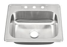
**457-4** Stainless Steel Top Mount Self Rimming Single Bowl Sink Material: T-304 Stainless Steel 18 Gauge Satin Finish Stone Guard Undercoated Overall Size: 25" x 22" x 8" Bowl Size: 21" x 15-3/4" x 8" Depth: 8" Sink Weight: 18 lbs. Template and Fastener Clips Included
