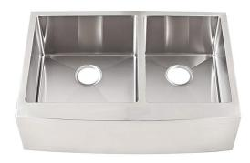
**437-UM-OS-FS** Stainless Steel Apron Double Bowl Undermount Sink Material: T-304 Stainless Steel 16 Gauge Satin Finish Stone Guard Undercoated Overall Size: 35-3/8" x 22-1/4" x 10" Left Bowl Size: 18-1/8" x 17-7/8" x 10" Right Bowl Size: 14" x 17-7/8" x 10" Depth: 10" Sink Weight: 35 lbs. Template and Fastener Clips Included
