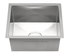
**450-HC-UM** Hand Crafted Stainless Steel Square Corner Single Bowl Undermount Sink Material: T-304 Stainless Steel 18 Gauge Satin Finish Stone Guard Undercoated Overall Size: 15-3/4" x 17-3/4" x 9" Bowl Size: 13-3/4" x 15-3/4" x 9" Depth: 9" Sink Weight: 25 lbs. Template and Fastener Clips Included
