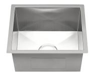
**20-250-5.5-UM** Square Corner Stainless Steel Single Bowl Undermount Sink Material: T-304 Stainless Steel 18 Gauge Satin Finish Stone Guard Undercoated Overall Size: 15-3/4" x 17-3/4" x 5-1/2" Bowl Size: 13-3/4" x 15-3/4" x 5-1/2" Depth: 5-1/2" Sink Weight: 20 lbs. Template and Fastener Clips Included
