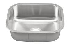
**458-UM** Undermount Stainless Steel Single Bowl Sink Material: T-304 Stainless Steel 18 Gauge Satin Finish Stone Guard Undercoated Overall Size: 23-3/8" x 17-3/4" x 9" Bowl Size: 21-3/8" x 15 3/4" x 9" Depth: 9" Sink Weight: 18 lbs. Template and Fastener Clips Included
