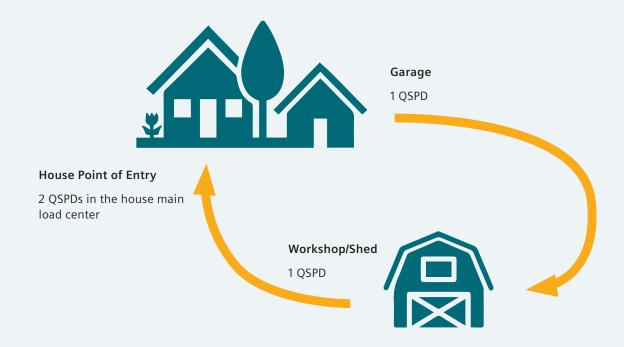
By installing 2 QSPDs in the house main load center at the point of entry, 1 unit in the garage, and 1 unit at the workshop or shed would provide overall more surge protection.
